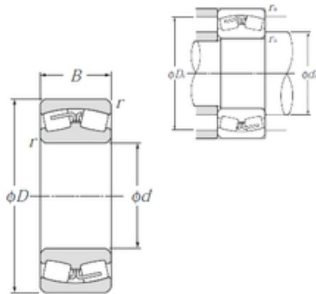
23138B Bearing 2D drawings and 3D CAD models
